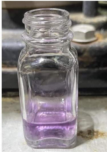
Figure 2: Reagent dissolved in sample water will turn purple
