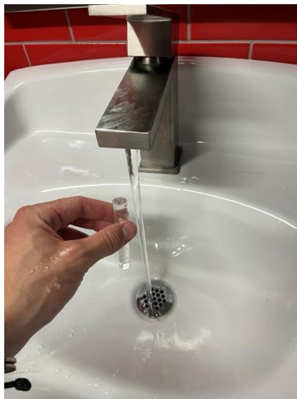
Figure 1: Rinse out the test tube and mixing bottle to remove any contaminants
