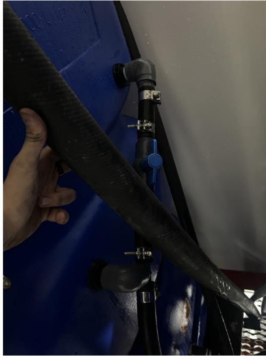
Figure 9: Final Fittings Assembly for Upper Jobe Float
