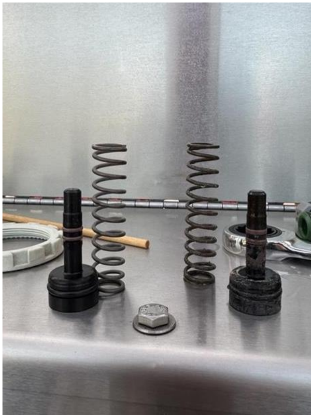
Figure 1 - New vs Old Hydrflex Cannon Plunger & Spring
