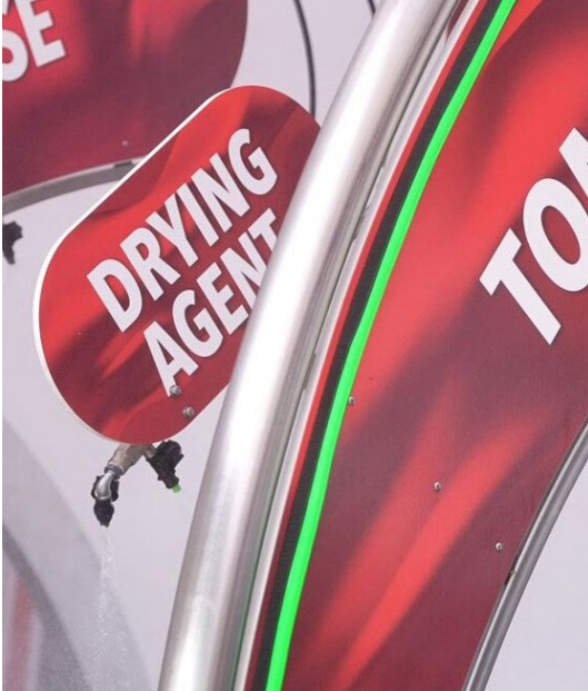
Figure 22: Drying Agent Manifold
