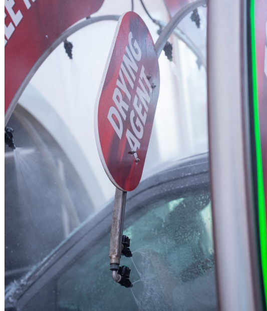
Figure 23: 10e40 Nozzles on Manifold side elbows
