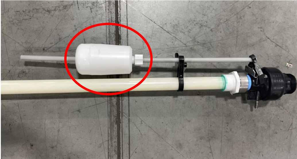
Figure 7 - Adjust the float approximately 4" to 5" from the end of the rod.
