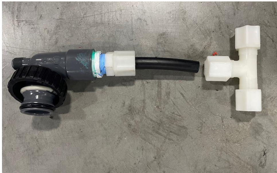
Figure 8 – Brine tank drain assembly; threaded plumbing adapter with 3/8" poly line installed. The plastic compression tee is added after plastic assembly has been installed in the brine tank. This plastic fitting will be on the exterior of the brine tank.
