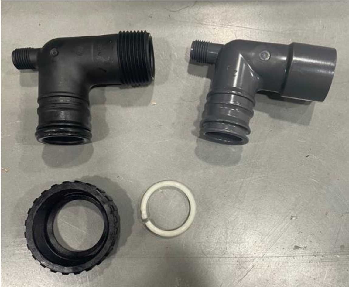
Figure 2 - Black piece on the left is what comes from the factory. Remove the snap ring, black threaded adapter, and O-ring. Install these on the grey part on the right.
