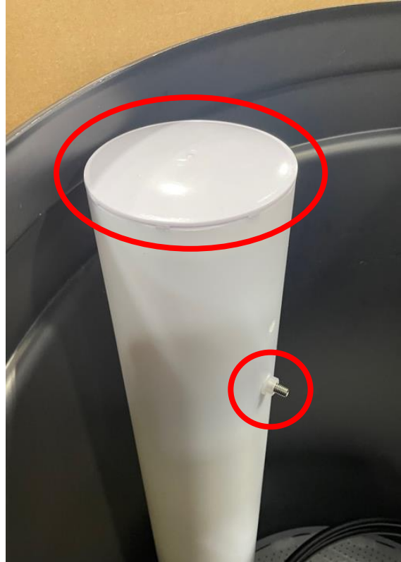
Figure 6 - Brine tank float. Remove the items circled in red PLUS the black threaded plumbing adapter sticking through the side of the brine tank.
