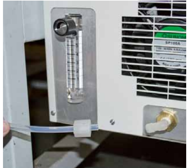
Flowmeter with O2 hose connected (left) Flowmeter with O2 hose disconnected @ 6 (right)
