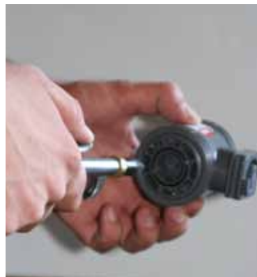
Valve and collar must line up before reattaching (top). Blowing compressed air through valve (left)
