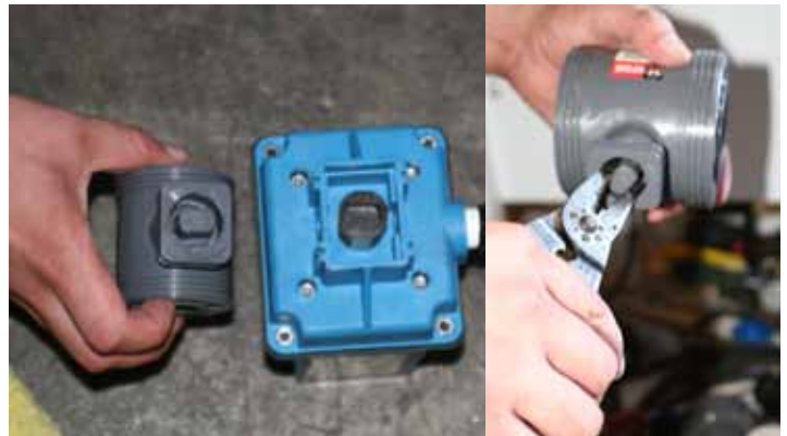
Valve and collar must line up before reattaching (top). Blowing compressed air through valve (left)
