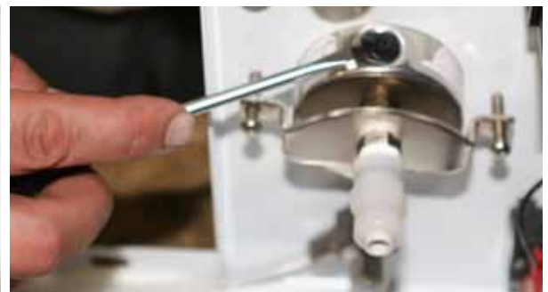
Venting the Ozone Pressure Gauge
